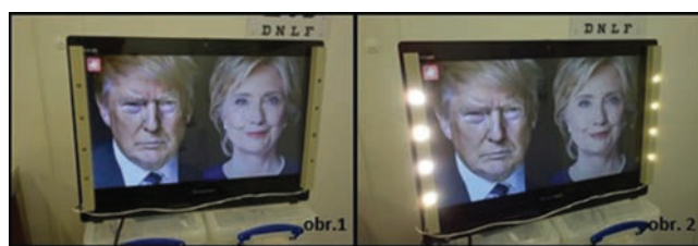
Fig. 2. Images designed for evaluation of subjective vision without and with glare
